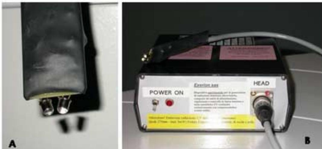
Figure 3: Left image (A) shows the Dresden modified Sierra Tip with double 370/10 UVA-Leads (Exerion Sas). In right image (B) the experimental electronic device for UVA leads alimentation (Exerion Sas).
